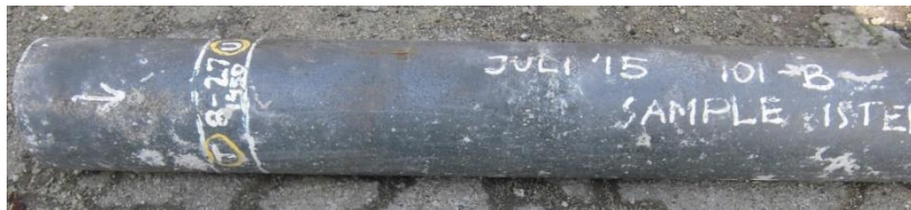
Gambar 11 Sampel tube reformer HP Nb Modified kondisi baik
